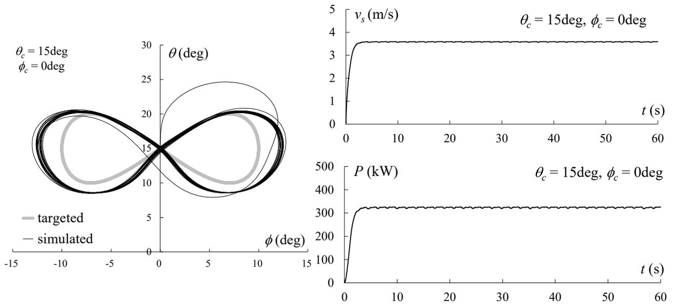
Fig. 7 Example of the simulation results in flight case of  $\theta_c = 15^\circ$ ,  $\phi_c = 0^\circ$
