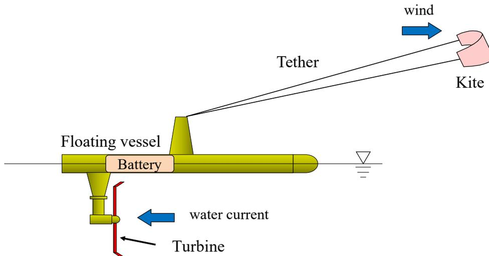
Fig. 2 The Autonomous Kite-Sailing Power Generation
