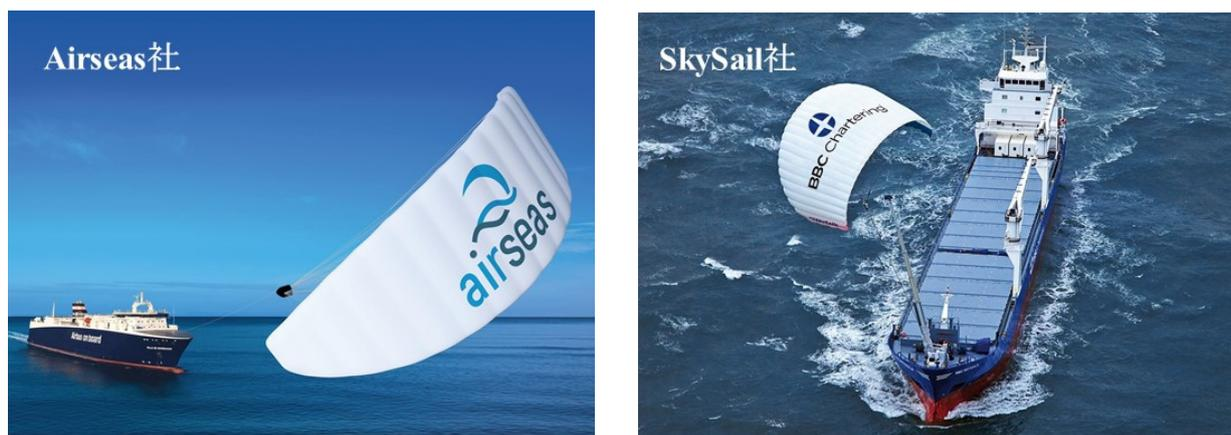
Fig. 4 Ship propulsion systems using towing kites<sup>5)6)</sup>
