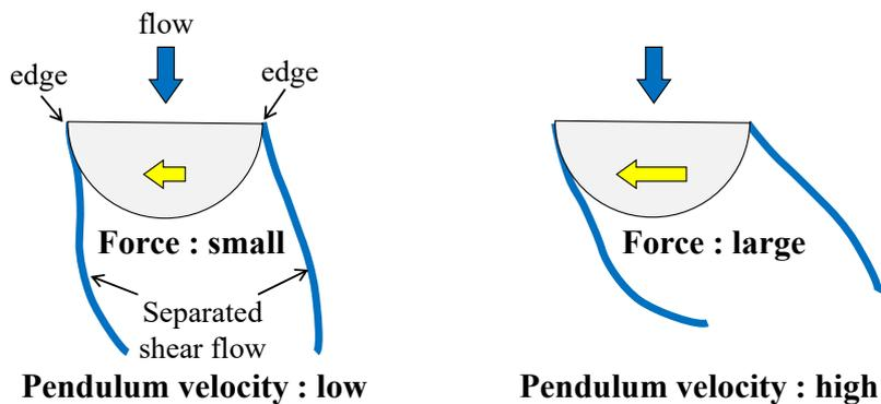
Fig. 9 Mechanism of galloping oscillation
