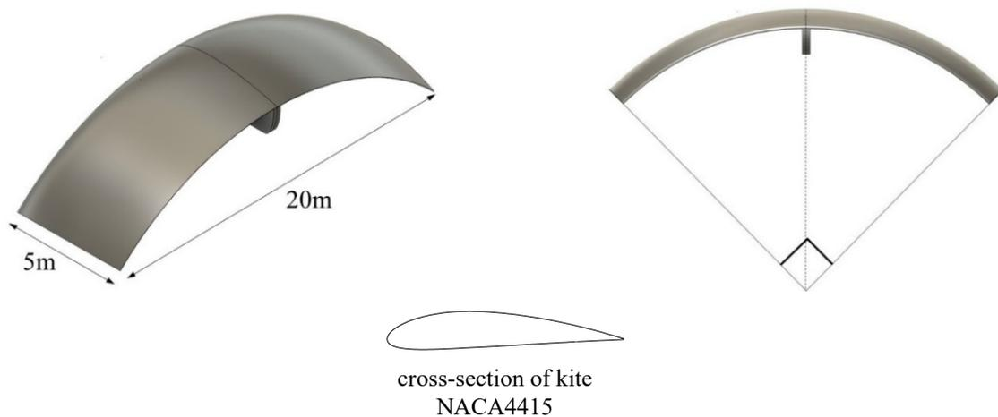
Fig. 5 Kite and its cross-section geometry used in the simulation
