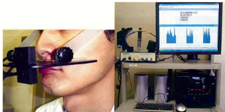
Fig 4. Nasometer II (KayPENTAX). Measure the ratio of sound pressure emitted from the nose in conversational speech.
