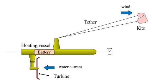
Fig. 2 The Autonomous Kite-Sailing Power Generation
