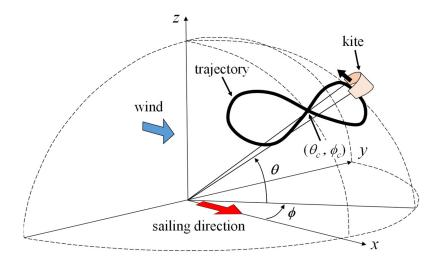
Fig. 6 Schematic of the simulation for the Autonomous Kite-Sailing Power Generation
