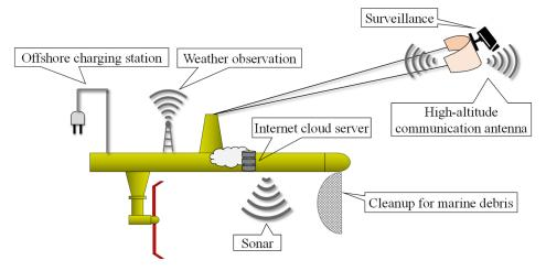
Fig. 3 The Autonomous Kite-Sailing Power Generation equipped with devices and sensors
