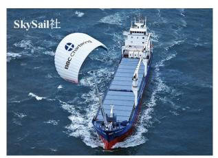
Fig. 4 Ship propulsion systems using towing kites<sup>5)6)</sup>
