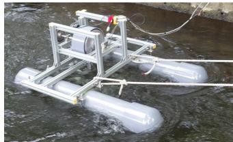
Fig. 11 Small-scale model of floating type turbine with the Hydro-VENUS rotor
