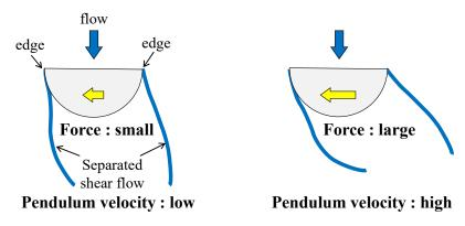
Fig. 9 Mechanism of galloping oscillation
