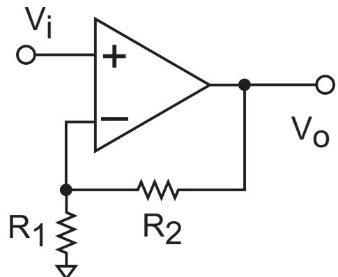
$$V^+ = V_i, \quad V^- = \frac{R_1}{R_1 + R_2} V_o$$
