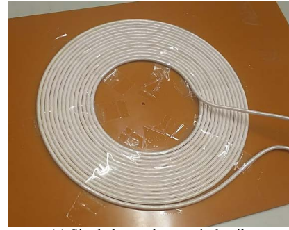
(a) Single layer planer spiral coil.
