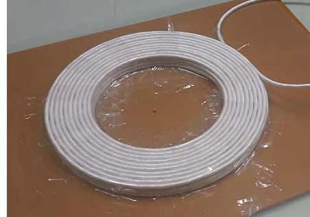
(b) multilayer planer spiral coil.
