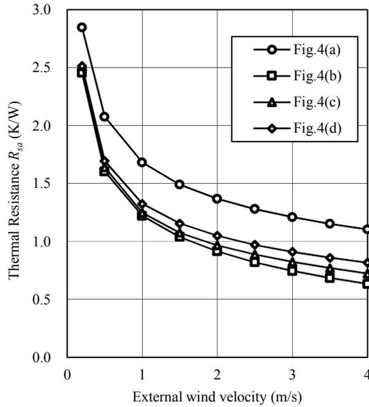
Fig. 6. Simulation results of the thermal resistance of the heat sink  $R_{sa}$ .
