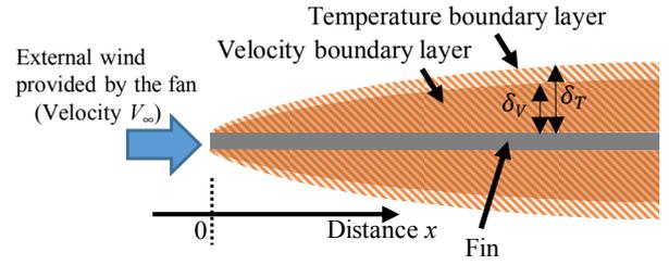
Fig. 2. Velocity and temperature boundary layer formed on a fin surface of the conventional heat sink structure by the external wind provided by the fan. (Horizontal sectional view)
