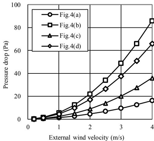
Fig. 11. Simulation results of the pressure drop by the heat sink.
