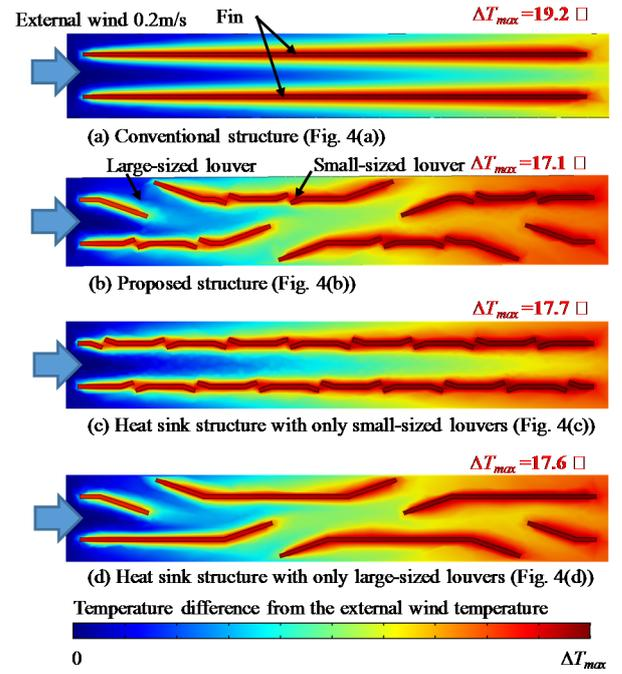
Fig. 7. Temperature difference of the air and fins from the external wind in the horizontal cross-section of the model space when the external wind velocity was set at 0.2m/s. For each model, the temperature difference is normalized by the maximum temperature difference in the cross-section ( $\Delta T_{max}$ ).
