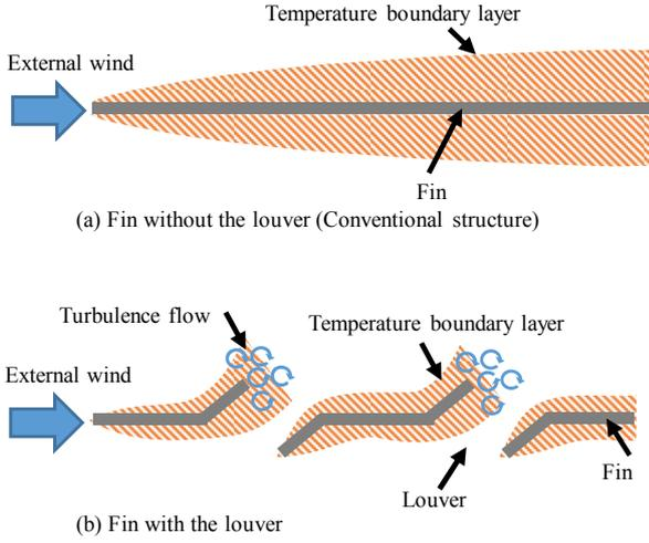
Fig. 3. Temperature boundary layer formed on a fin with and without the louvers. (Horizontal sectional view)
