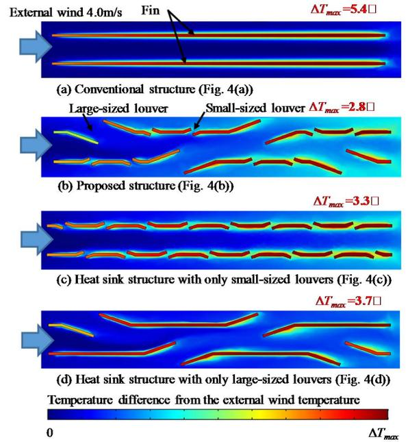
Fig. 8. Temperature difference of the air and fins from the external wind in the horizontal cross-section of the model space when the external wind velocity was set at 4.0m/s. For each model, the temperature difference is normalized by the maximum temperature difference in the cross-section ( $\Delta T_{max}$ ).
