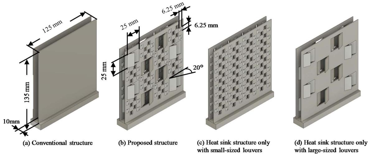
Fig. 4. Simulation models of the 4 types of the heat sinks.
