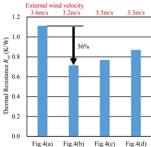
Fig. 12. Estimation result of the thermal resistance of the heat sinks provided with the external wind using the commercial DC fan.
