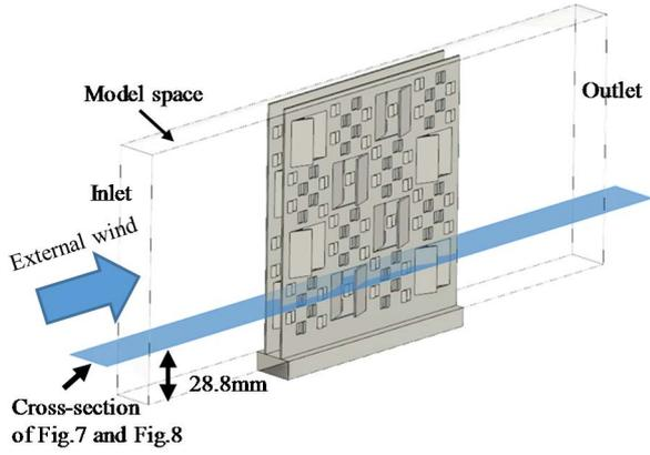
Fig. 9. Horizontal cross-section taken for Fig. 7 and Fig. 8.
