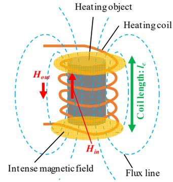
Fig. 2. Magnetic flux lines around conventional heating coil structure.
