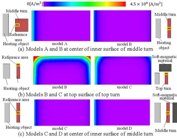
Fig. 8. Simulated current density distribution in heating coil wire cross-section.
