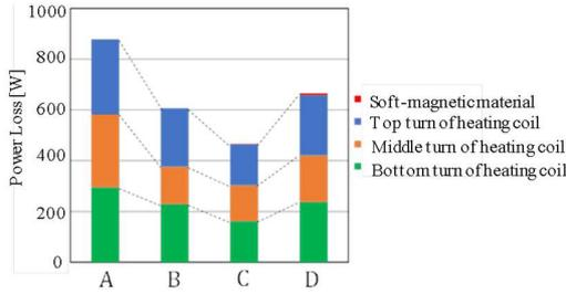
Fig. 7. Simulated power loss breakdown of heating coil structure.
