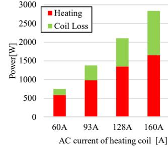
Fig. 12. Estimation result of heat generation and coil loss of prototype of proposed heating coil structure.
