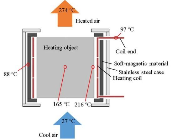
Fig. 11. Measurement points and results of temperature in prototype of proposed heating coil structure. Temperature was observed immediately after ac current of 160 Arms at 400 kHz was applied to heating coil for 3 minutes. Heating coil, soft-magnetic material, and stainless steel case were thermally isolated each from others using glasswool.
