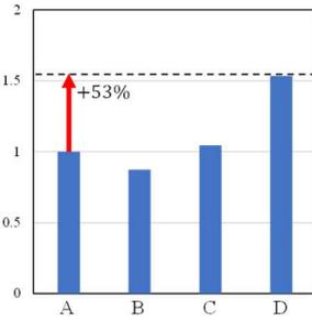
Fig. 6. Squared magnetic field intensity averaged over heating object normalized by that of model A.
