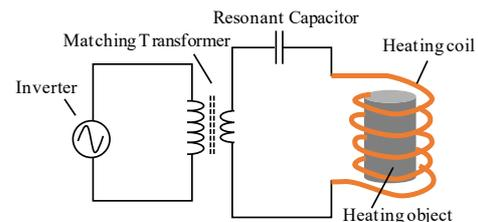
Fig. 1. Induction heating system with conventional heating coil structure.
