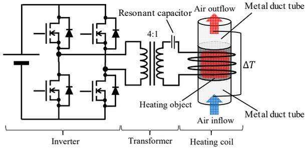
Fig. 10. Experimental circuit of proposed heating coil structure.
