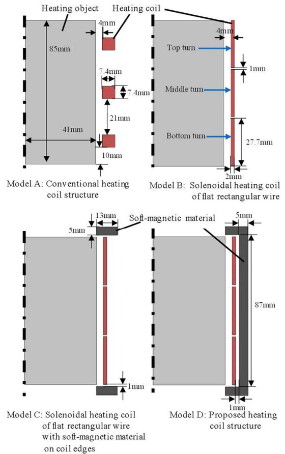
Fig. 4. Cross-section view of simulation models.
