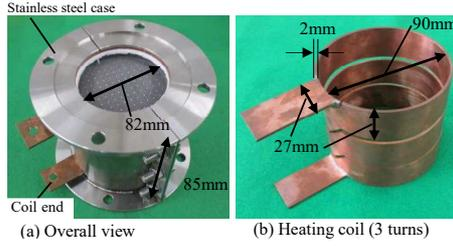
Fig. 9. Experimental circuit of proposed heating coil structure.
