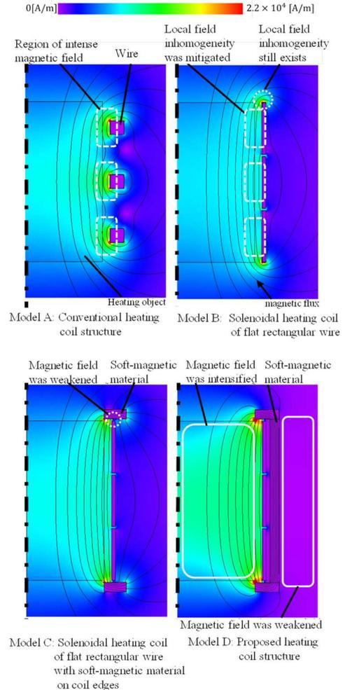
Fig. 5. Simulated magnetic field distribution.
