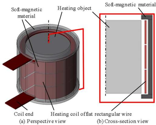
Fig. 3. Proposed heating coil structure.
