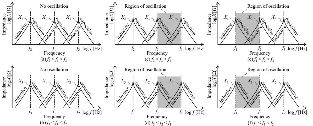
Fig. 5 Frequency region of the oscillation in 6 possible magnitude relation among  $f_1$ – $f_3$ . The vertical and horizontal axes are the impedance of  $N_1$ – $N_3$  and the frequency, respectively, both in the logarithmic scale.
