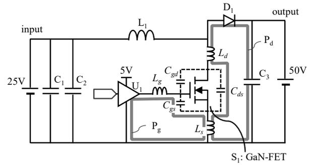
Fig. 1. Circuit diagram of the experiment boost chopper.
