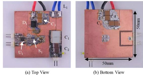
Fig. 2. Photographs of the experimental chopper.
