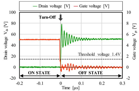
Fig. 10. Voltage waveforms at the turn-off when the oscillatory false triggering does not occur.
