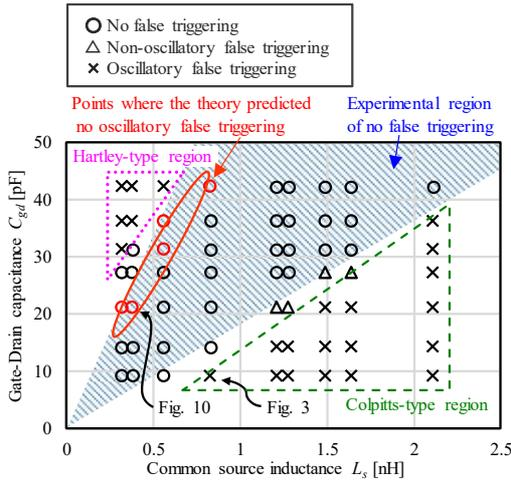
Fig. 9. Experimental result of occurrence of the oscillatory false triggering. Red marks indicate the points where the theory predicted non-occurrence of the oscillatory false triggering.
