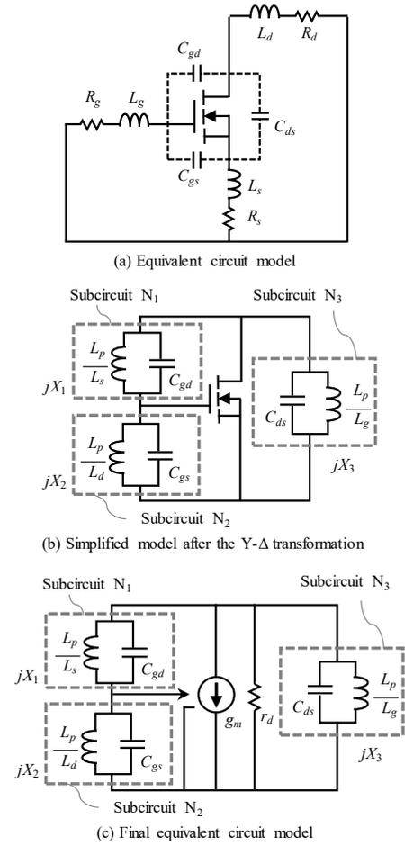
Fig. 4. Analytical models of the oscillatory false triggering.
