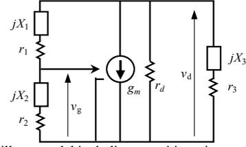
Fig. 12. Oscillator model including parasitic resistance.
