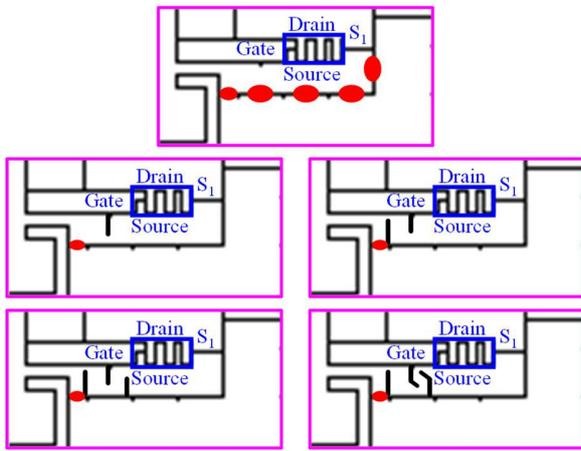
Fig. 7. Nine variations in the common source paths. Red points show the points for making a solder bridge.
