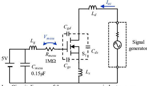
Fig. 11. Circuit diagram of the common source inductance measurement system.
