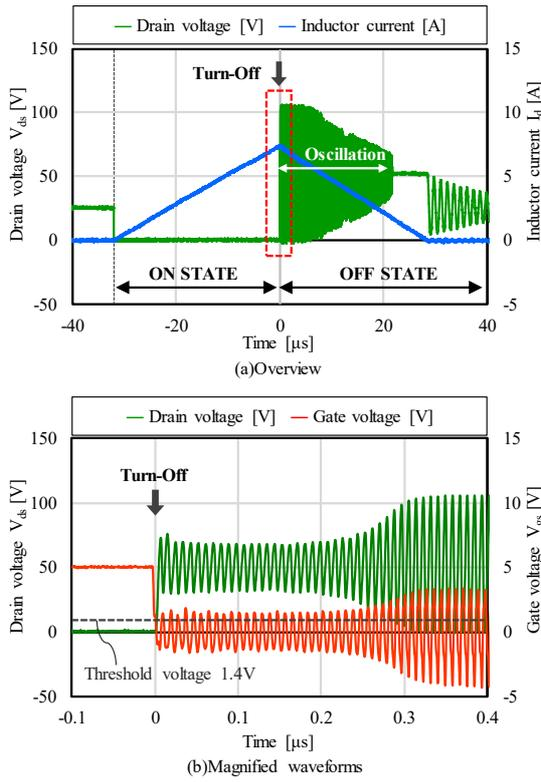
Fig. 3. Experimental waveforms after the turn off.
