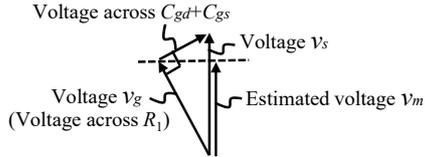
Fig. 5. Phasor diagram of the voltage induced in the common source inductance.
