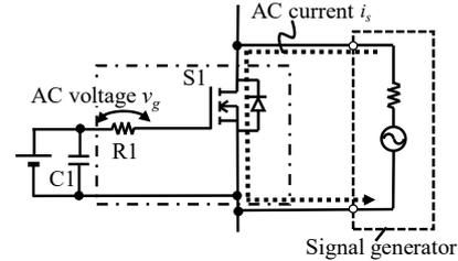
Fig. 1. Schematic diagram of the proposed method applied to a switching device under test.
