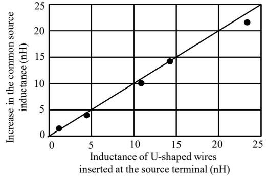
Fig. 13. Dependence of the measured increase in the common source inductance on the inductance of U-shaped wires.
