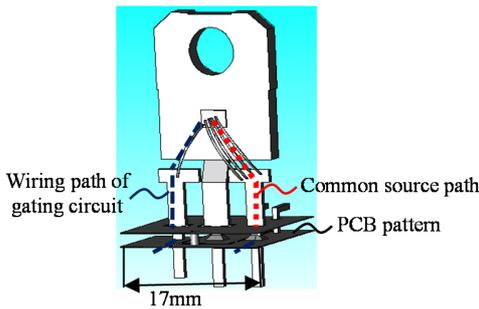
Fig. 10. Simulation model of PCB A with the semiconductor package mounted on-board.
