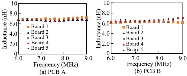
Fig. 9. Measurement results of the common source inductance.
