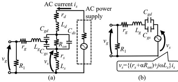
Fig. 4. Modified AC equivalent circuit of Fig. 3(b) including resistor R1.
