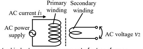
Fig. 2. Mutual inductance measurement of a transformer.
