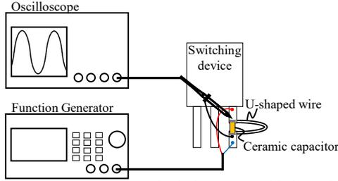
Fig. 12. Measurement system of the inductance of U-shaped wires.
