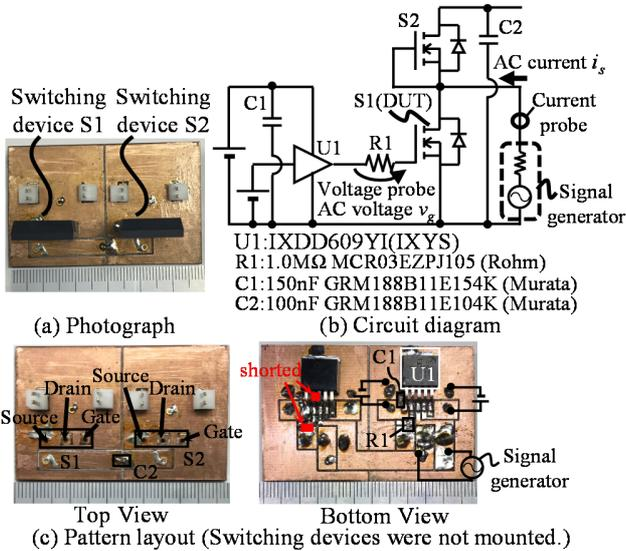
Fig. 7. Experimental PCB of a half-bridge circuit (PCB B).
