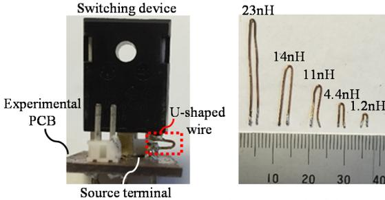
Fig. 11. U-shaped wires inserted at the source terminal of the semiconductor package mounted on PCB A.
