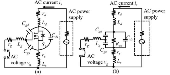
Fig. 3. AC equivalent circuit model of the mutual inductance measurement method applied to the common source inductance.
