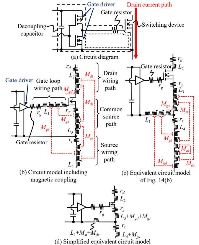
Fig. 14. Simple circuit model of a switching device with a gate driver.
