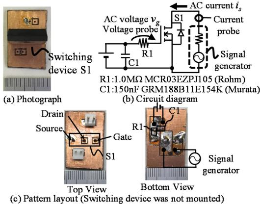
Fig. 6. Experimental PCB only with a switching device (PCB A).
