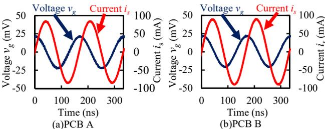
Fig. 8. Measurement results of the voltage and current waveforms.
