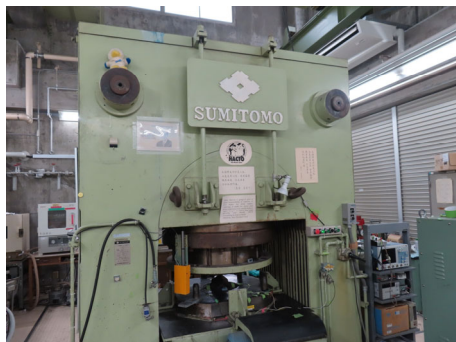
一軸加圧式川井型超高压発生装置 USSA-5000/KAWAI-type multi- anvil high-pressure apparatus, USSA-5000
