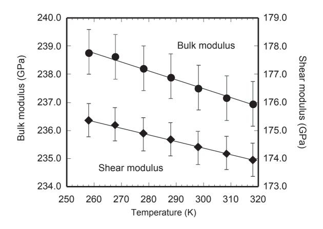
Figure 3. Adiabatic bulk and shear moduli of  $MgSiO_3$  perovskite as a function of temperature. The relatively large errors resulted from uncertainty of the diameter.
