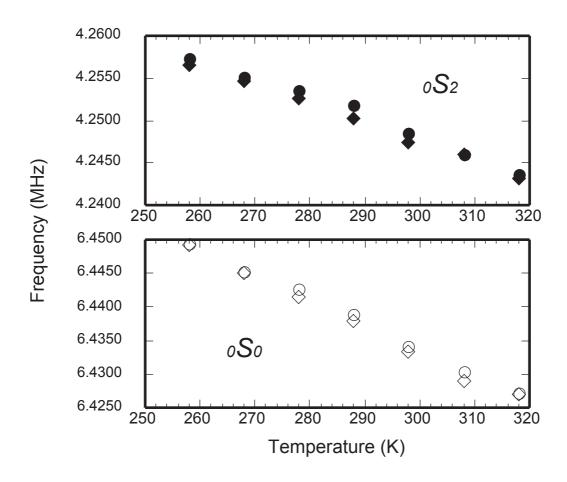
Figure 2. Temperature dependence of resonant frequencies of MgSiO<sub>3</sub> perovskite for  $_0S_0$  and  $_0S_2$  resonant modes. The temperature was controlled within 0.1 K during the measurements at 10 K intervals. The circles and diamonds represent the heating and cooling processes, respectively.
