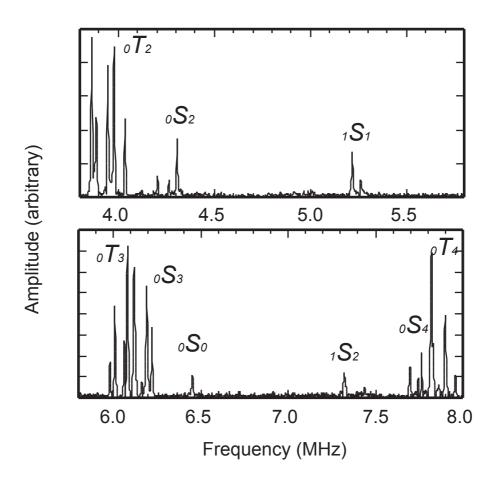
Figure 1. An example of resonant spectra at 258 K. Data was obtained at 100Hz intervals.
